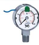
Contact gauge with inductive contact (KI), for visual and acoustic warning of low gas supply pressure and to monitor the cylinder pressures; for inert, combustible, oxidizing and corrosive gases and gas mixtures, nominal pressure maximum 300 bar
